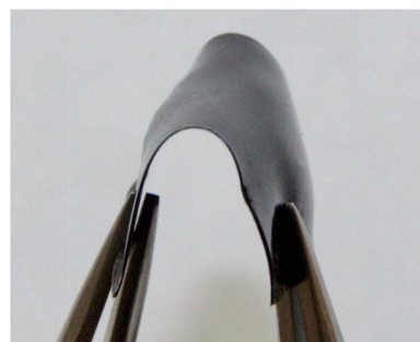
Fig. 5 Photograph of film F2 after reaction at 200 °C. The image shows the film flexed between pairs of tweezers at room temperature.
