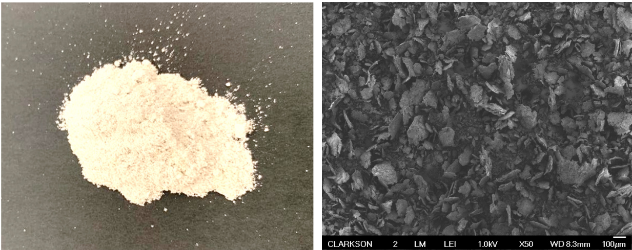
FIGURE S5 (a) Photograph of a composite powder prepared by low-energy blending of PEEK (70 wt %) and hBN (30 wt %), and (b) its SEM image. The smaller particles are hBN, and the larger ones are flattened PEEK.
