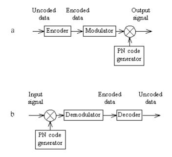
Figure 1: Simplified block diagram of the data processing structure: (a) transmitter part, (b) receiver part.
