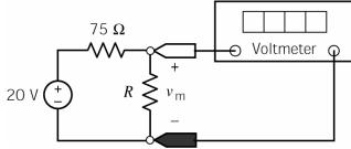
The resistor represents a temperature sensor. Suppose the resistance R, in  $\Omega$ , is related to the temperature T, in  ${}^{\circ}$ C, by the equation
