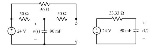
After replacing series and parallel resistors by equivalent resistors, the part of the circuit connected to the capacitor is a Thevenin equivalent circuit with  $R_t = 33.33 \Omega$ . The time constant is  $\tau = R_t C = 33.33 (0.090) = 3 \text{ s}$ .
