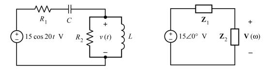
Given that  $\mathbf{Z}_1 = 15.3 \angle -24.1^{\circ} \Omega$ ,  $\mathbf{Z}_2 = 14.4 \angle 36.9^{\circ} \Omega$  and  $\mathbf{V}(\omega) = A \angle 31.5^{\circ} V$ , determine the values of A,  $R_1$ ,  $R_2$ , L and C.
