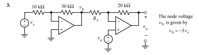
The input to this circuit is the voltage  $v_s$ . The output is the node voltage  $v_o$ . The output is related to the input by the equation  $v_o = m v_s + b$  where *m* and *b* are constants.
