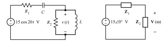
Given that  $\mathbf{Z}_1 = 15.3 \angle -24.1^\circ \Omega$ ,  $\mathbf{Z}_2 = 14.4 \angle 36.9^\circ \Omega$  and  $\mathbf{V}(\omega) = A \angle 31.5^\circ V$ , determine the values of A,  $R_1$ ,  $R_2$ , L and C.
