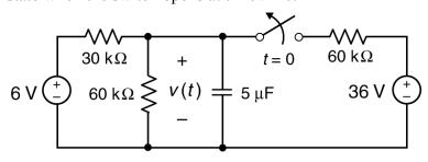
The capacitor voltage is  $v(t) = A + Be^{-at}$  for  $t \ge 0$ . Determine the values of the constants A, B, and a:
