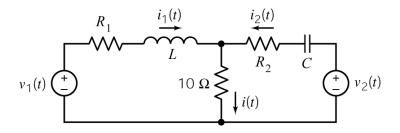
This circuit is at steady state. The voltage source voltages are given by
