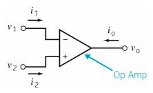
• The simplest model of the op amp, and the only model that we will use in this course, is the ideal op amp. The input currents of an ideal op amp are zero and the input voltages are equal.
