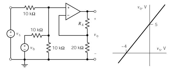
The input to this circuit is the voltage,  $v_s$ . The output is the voltage  $v_o$ . The voltage  $v_b$  is used to adjust the relationship between the input and output. Determine values of  $R_4$  and  $v_b$  that cause the circuit input and output have the relationship specified by the graph
