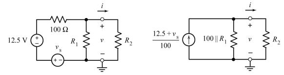
Recognizing the parameters of the Norton equivalent circuit gives:
