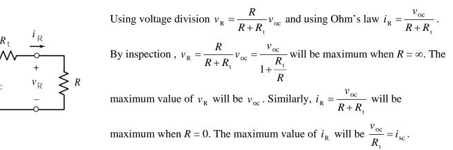
The maximum power transfer theorem tells use that  $p_{\rm R} = i_{\rm R} v_{\rm R}$  will be maximum when  $R = R_{\rm t}$ . Then
