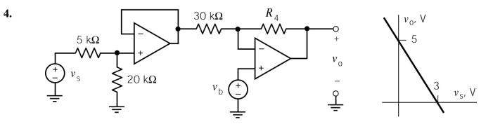
The input to this circuit is the voltage,  $v_s$ . The output is the voltage  $v_o$ . The voltage  $v_b$  is used to adjust the relationship between the input and output. Determine values of  $R_4$  and  $v_b$  that cause the circuit input and output have the relationship specified by the graph
