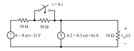
Determine  $v_0(1)$ ,  $v_0(3)$ ,  $v_0(5)$ , and  $v_0(7)$ ; the values of the voltage  $v_0(t)$  at times t = 1, 3, 5 and 7 seconds.
