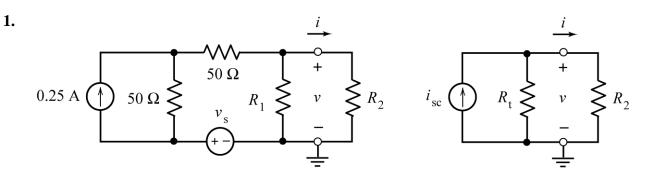
The part of the first circuit to the left of the terminals can be reduced to its Norton equivalent circuit using source transformations and equivalent resistance. The resulting Norton equivalent circuit will be characterized by the parameters:
