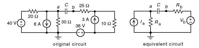
The equivalent circuit on the right is obtained from the original circuit on the left using source transformations and equivalent resistances. (The lower case letters a and b identify the nodes of the capacitor in both the original and equivalent circuits.) Determine the values of  $R_a$ ,  $I_a$ ,  $R_b$  and  $V_b$  in the equivalent circuit:
