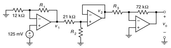
The values of the node voltages  $v_1$ ,  $v_2$  and  $v_0$ , are  $v_1 = 875$  mV,  $v_2 = 350$  mV and  $v_0 = -600$  mV. Determine the value of the resistances  $R_1$ ,  $R_2$  and  $R_3$ :
