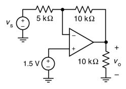
**3.** Here's a circuit and its Thevenin equivalent circuit. Determine the values of the Thevenin resistance,  $R_{\rm t}$ , and of the open-circuit voltage,  $V_{\rm oc}$ .
