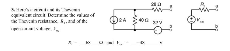
**4.** Here's a circuit and its Thevenin equivalent circuit. Determine the values of the Thevenin resistance,  $R_t$ , and of the open-circuit voltage,  $V_{oc}$ .
