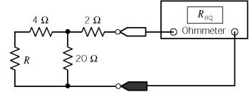
The Ohmmeter measures equivalent resistance.
