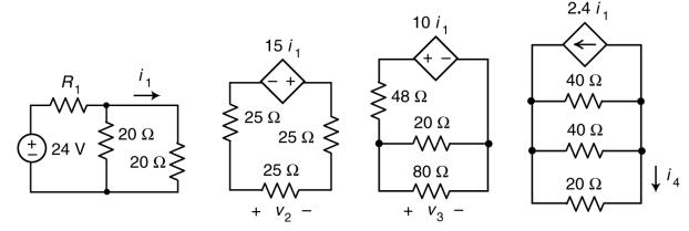
Here's a single circuit drawn in four parts for convenience. The four parts are connected by the dependent sources. Given that  $i_1 = 0.8$  A, determine the values of  $R_1$ ,  $v_2$ ,  $v_3$ , and  $i_4$ .
