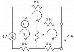
Let  $i_1$ ,  $i_2$  and  $i_3$  denote the mesh currents in meshes 1, 2 and 3, respectively.
