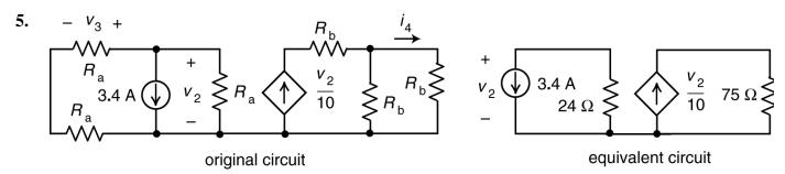
The equivalent circuit on the right is obtained from the original circuit on the left by replacing series and parallel combinations of resistors by equivalent resistors. The original circuit contains 3 equal resistances labeled  $R_{\rm a}$  and another 3 equal resistances labeled  $R_{\rm b}$ . Determine the values of  $R_{\rm a}$  and  $R_{\rm b}$ . Given that
