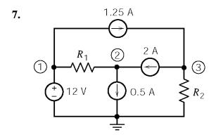
The encircled numbers are node numbers. The corresponding node voltages are
