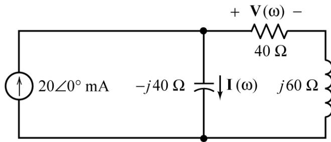
$$\mathbf{I}(\omega) = \frac{40 + j60}{-j40 + (40 + j60)} \times 0.020\angle 0^\circ = 24.25\angle 50.9^\circ \text{ mA}$$
