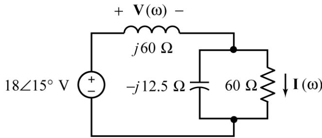
$$\mathbf{V}(\omega) = -\frac{j60}{j60 + (-j12.5 \parallel 60)} \times 18\angle 15^\circ = \frac{(60\angle -90^\circ)(18\angle 15^\circ)}{j60 + \frac{60(-j12.5)}{60 - j12.5}} = 22.46\angle 18^\circ \text{ V}$$
