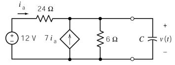
Represent the capacitor voltage v(t) as a function of t for  $t \ge 0$ .
