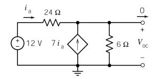
$$i_{a} = \frac{12 - V_{oc}}{24} \cdot \text{Then} (7+1) \left(\frac{12 - V_{oc}}{24}\right) = \frac{V_{oc}}{6}$$
