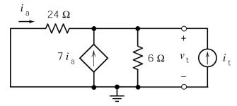
$$i_{a} = -\frac{v_{t}}{24} \cdot \text{Then } i_{t} + 7\left(-\frac{v_{t}}{24}\right) = \frac{v_{t}}{24} + \frac{v_{t}}{6}$$
