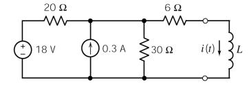
Represent the inductor current i(t) as a function of t for  $t \ge 0$ .
