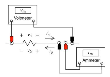
Suppose  $v_{\rm m} = 12$  V and  $i_{\rm m} = -2$  A. The value of power dissipated by the resistor is \_\_\_\_\_ W.
