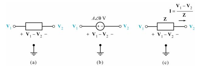
We can express the (a) element voltage, (b) source voltage or (c) current and/or voltage of an impedance in terms of node voltages.
