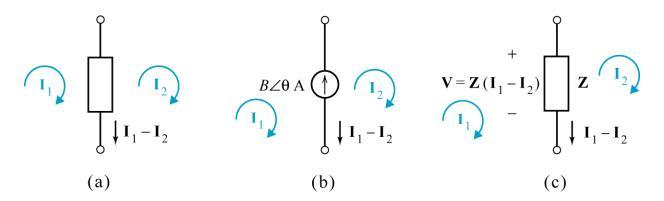
We can express the (a) element current, (b) source current or (c) current and/or voltage of an impedance in terms of mesh currents.
