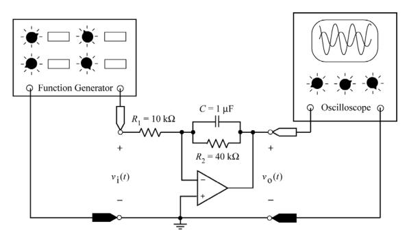
Here a function generator provides the input to a linear circuit and the oscilloscope displays the output, or response, of the linear circuit. The function generator allows us to choose from several types of input function.
