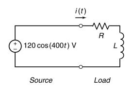
**b)** Suppose **instead** that  $i(t) = 191\cos(400t - 37.2^{\circ})$  mA. Determine the values of the real and reactive powers supplied by the source to the load.
