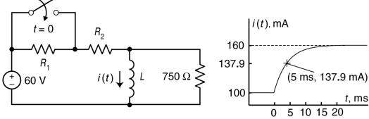
Determine the values of  $R_1$  and  $R_2$ .
