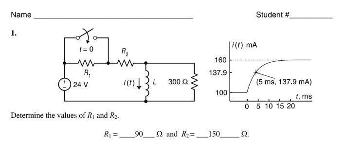
**b.** Determine the value of the time constant,  $\tau$ , of the this circuit after the switch closes:  $\tau = 5$  ms.
