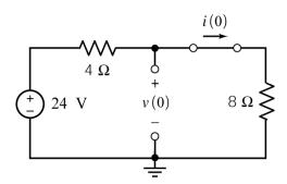
**9.** Given that  $\mathcal{L}[v(t)] = \frac{a s + b}{2 s^2 + 40 s}$  where v(t) is the voltage shown to the right, determine the values of a and b.
