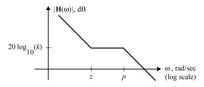
Determine the values of the constants k, z and p used to label the Bode plot:
