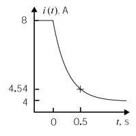
Here's a plot of the inductor current. Determine the values of D and E used to represent the circuit in the complex frequency domain:
