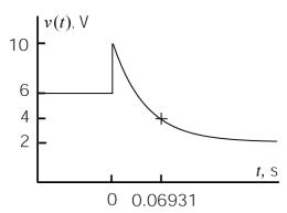
From the plot, v(0+) = 10 V and  $\lim_{t \to \infty} v(t) = 2 \text{ V}$ . From the final value theorem,
