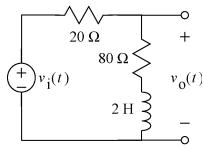
The values of the corner frequencies are  $z = \underline{\phantom{a}} 40\underline{\phantom{a}}$  rad/sec and  $p = \underline{\phantom{a}} 50\underline{\phantom{a}}$  rad/sec.
