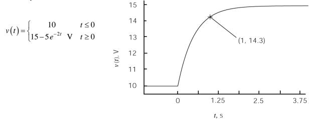
One more observation, eventually the transient part of the response dies out and the circuit reaches steady state. It is, once again, a dc circuit. The capacitor acts like an open circuit, so we have
