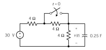
Determine the voltage, v(t), for this circuit.
