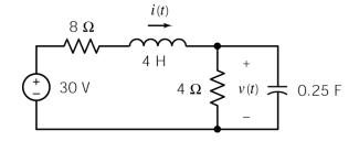
Determine the current, i(t), and voltage, v(t), for this circuit.
