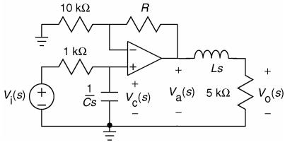
We can save ourselves some work be noticing that the 10000 ohm resistor, the resistor labeled R and the op amp comprise a non-inverting amplifier. Thus
