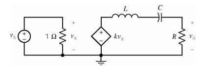
The input of this circuit is the voltage source voltage,  $v_{\rm s}$ . The output is the resistor voltage,  $v_{\rm o}$ . Design this circuit to have the step response
