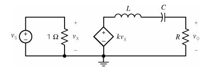
The input of this circuit is the voltage source voltage,  $v_s$ . The output is the resistor voltage,  $v_o$ . Design this circuit to have the step response
