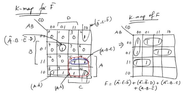
$A = A = A + \overline{B}$  to avoid static-o hoggerd. Thus,  $\overline{F} = (A \cdot \overline{B}) + (A \times B \cdot C) + (\overline{B} \cdot C - \overline{D}) + (\overline{A} \cdot \overline{B})$   $(\overline{C} \cdot D) + (A \cdot C)$  $\overrightarrow{F} = (\overline{A} + B) \cdot (B + \overline{C} + D) \cdot (A + \overline{B} + C + \overline{D}) \cdot (\overline{A} + \overline{C})$
