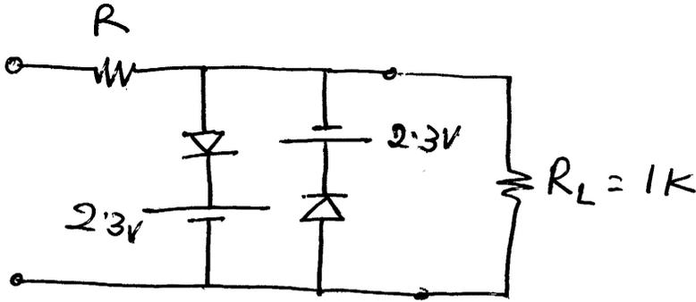
2.3V power supplies are used to provide  $\pm 3V$  limiting levels
