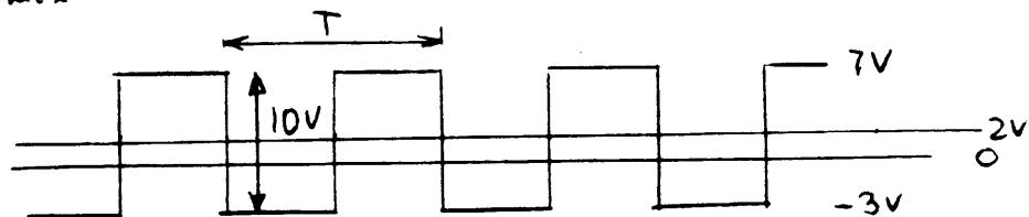
Diode still conducting for half the cycle ( $T/2$ )
