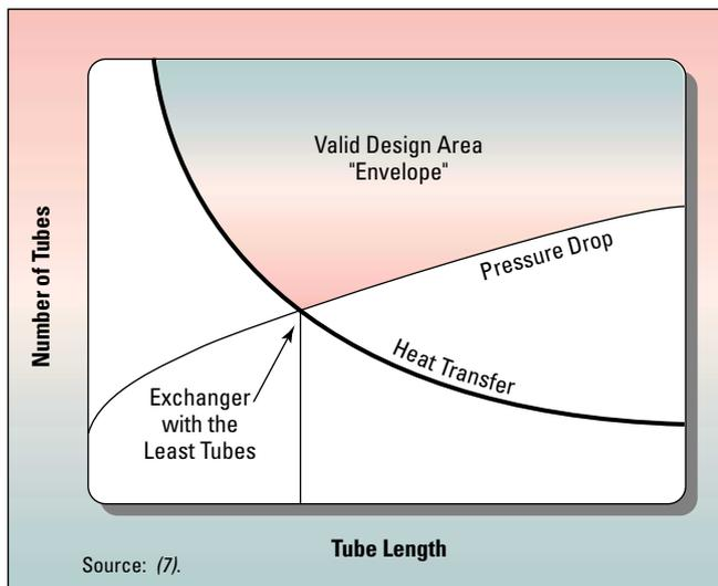
■ Figure 4. Envelope curve for a clean exchanger.
