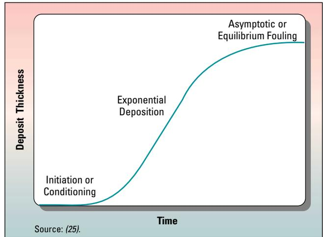
Figure 1. Idealized fouling curve.
