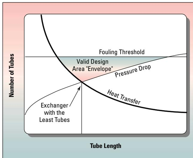
■ Figure 5. Envelope curve with fouling in mind.
