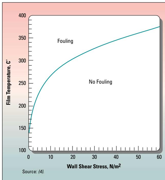
Figure 3. Threshold film temperature as a function of wall shear.
