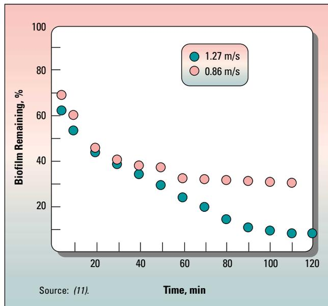
Figure 6. The effect of velocity on the effectiveness of chlorine as a biocide at a concentration of 6.3 mg/L for the removal of biofilms.
