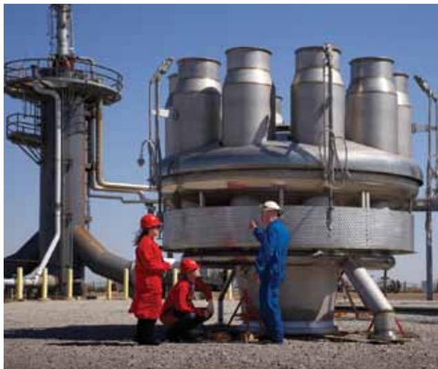
▲ **Figure 8.** An advanced steam-assisted flare tip (before mounting on a flare stack) improves smokeless performance.
