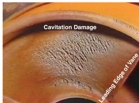
◀ **Figure 6.** Cavitation damage has occurred on an impeller. Source: The Hydraulic Institute, Inc.
