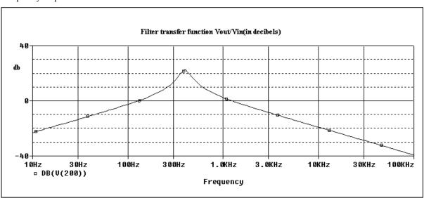
7. On the graph, mark the upper and lower 3db points, and determine the bandwidth of the filter.
