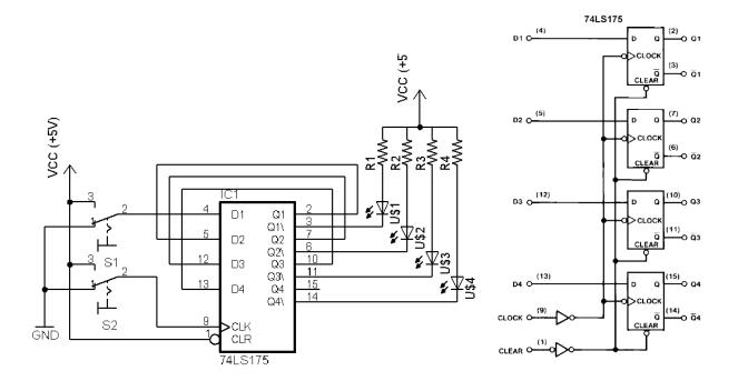
The circuit above is exactly the same as you had in "Sequential circuits" lab. To remind you of the functionality provided by the TTL chip 74LS175, its logic diagram is given on the right.
