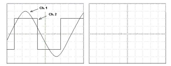
1. For the trace above, original scope settings are: time base 1 usec/div, vertical scale 1V/div, center line is at 0V, triggering from Ch.1 at the level of -0.8V, positive slope. Redraw the traces in the provided space, given that triggering is switched to Ch.2.
