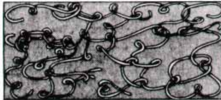
(b) Schematic of oriented amorphous polymer
