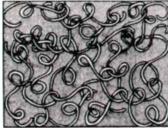
(a) Schematic of unoriented amorphous polymer
