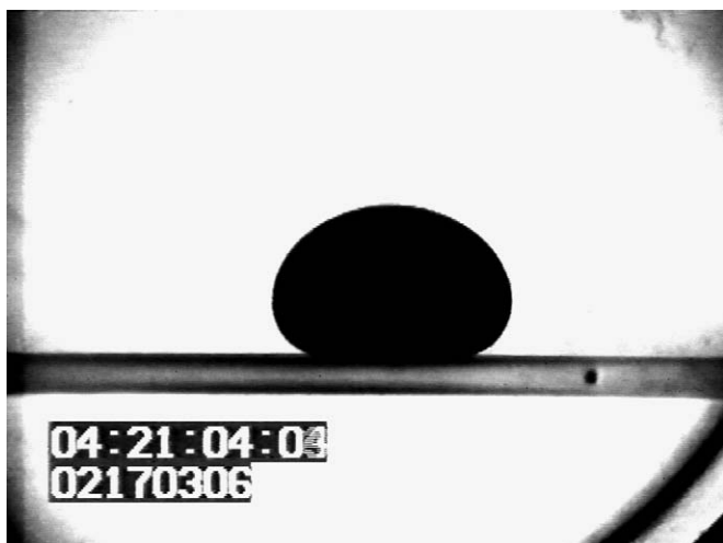
Fig. 3. Image of a drop grabbed from a videotape of an experiment on Ga-doped InSb in Ar and 2.0 \times 10^{-7} bar O_2 . Note that there is no reflection of the drop on the substrate surface, indicating that the camera is properly aligned with the substrate.
