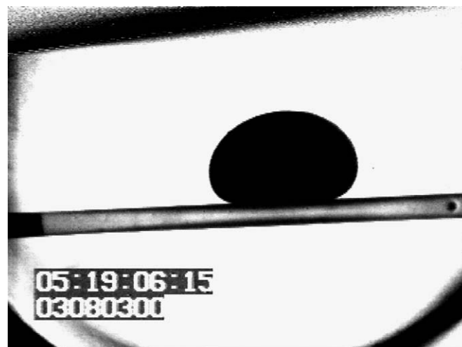
Fig. 4. Image of a drop on a tilted substrate from an experiment on Ga-doped InSb in Ar and 2.8 \times 10^{-7} bar O_2 . This image was grabbed just before the drop rolled down the substrate.
