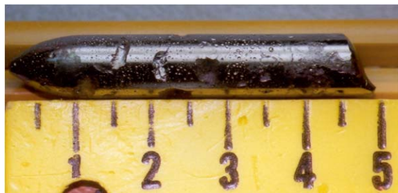
Fig. 5. Photograph of Ingot 19 showing attached regions with small bubble voids and large cavities.
