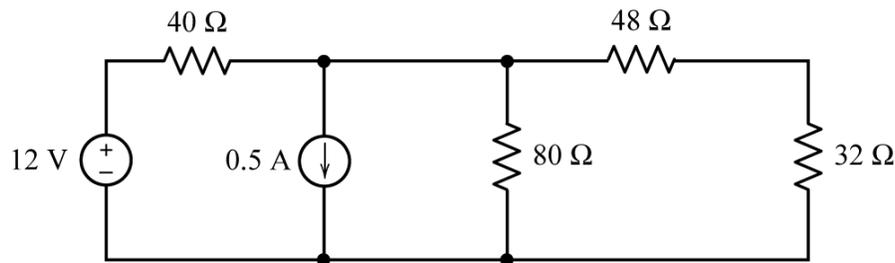
Label the resistor voltages and currents. In anticipation of using Ohm's law, label the voltage and current of each resistor to adhere to the passive convention.
