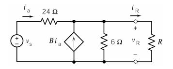
Solution: We can replace the part of the circuit to the left of the terminals by its Thevenin equivalent circuit:
