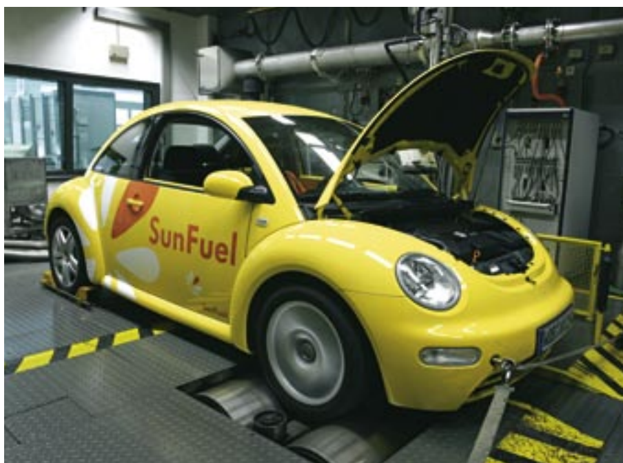
Powering up for a better climate: Measuring emissions from a SunFuel-powered New Beetle on a rolling-road test rig
