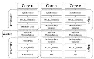
Figure 2 Controller-Helper Design Pattern
