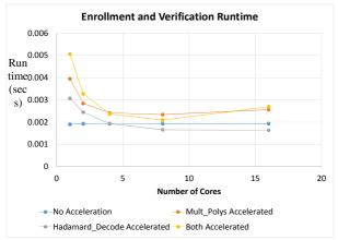
**Figure 6 Enrollment and Verification Runtimes at** 875 MHz
